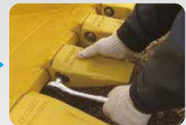
Set bushing, washer and bolt and tighten by a ratchet wrench.
